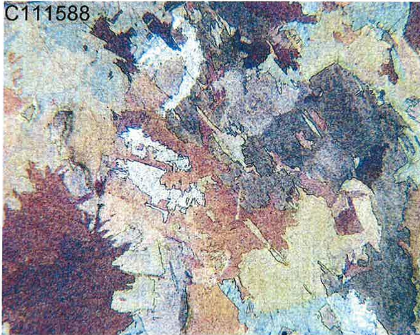
Fig. 3. Weld metal, fusion line and the heat affected zone. Magnification: 100 X.
