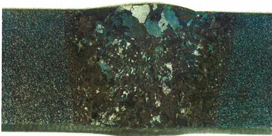
Fig.1. Macrograph of etched cross section of the welded joint. Magnification: 4 X.
